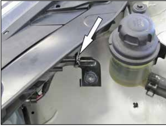
7. Remove the factory air box mounting bracket shown from the back of the headlight.
