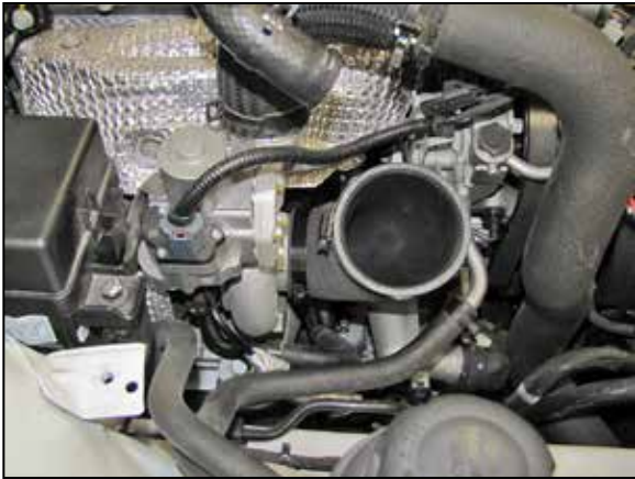
8. Install the provided elbow hose (08504) onto the turbo inlet and secure with the provided hose clamp.
