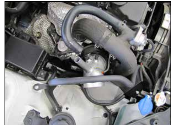
18. Install the K&N® intake tube into the heat shield and silicone hose then adjust the hose and tube for best fit and secure with the provided hose clamps.
